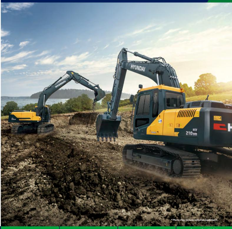
**Gross Power** 148 HP(110 kW) at 2,000rpm
