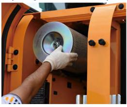
Electric control box and Air cleaner are centralized in one or the same compartment for easy service.
