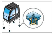
The application of Viscous Mounting to the cabin support provides the operator with a much improved ride. The operator work efficiency will increase as the shock and noise level in the cabin decreases.
